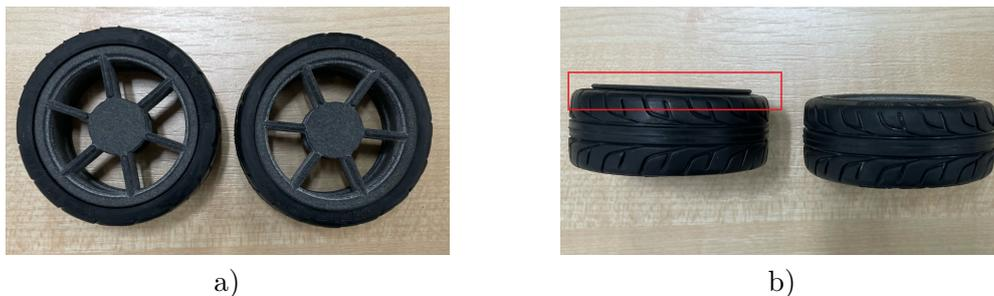
**Figure 2.7.** Example of an insufficient assembly of a wheel, which is undetectable by the camera-based method. In the subfigure a), the wheels look assembled correctly, but the side view in subfigure b) shows that one wheel is assembled correctly and the other poorly. The fault is highlighted in the red rectangle.
