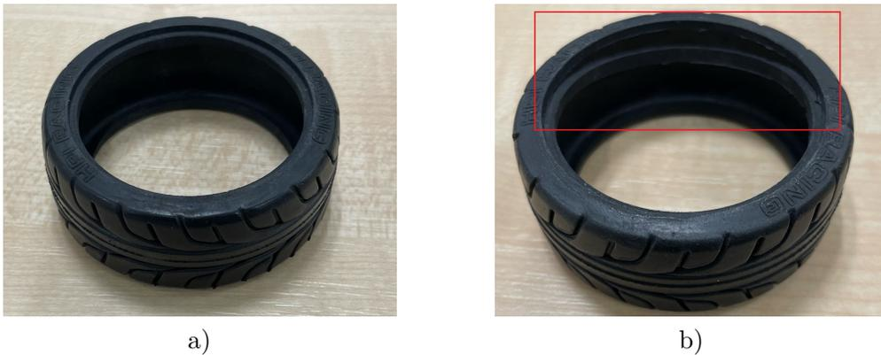
**Figure 2.8.** Example of a normal and a defected tire. An undamaged tire should look like the one in the subfigure a). The rubber of the tire in the subfigure b) is torn on the inside of the tire which can be seen in the red rectangle.
