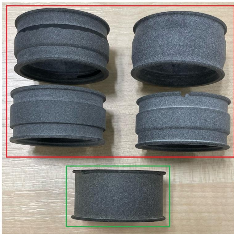
**Figure 2.10.** Examples of different defects on the rims used as anomalous data. The rims in the red rectangle are defective, the rim in the green rectangle is an example of a correctly manufactured rim.
