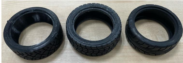
**Figure 2.9.** Tires of different stiffness used as anomalous data. The left tire is 3D printed and is very stiff, the tire in the middle is a different type of a tire and is a bit stiffer than the normal tire and the tire in the right is less stiff than the normal tire. The tire with normal stiffness can be seen in figure 2.8, subfigure a).
